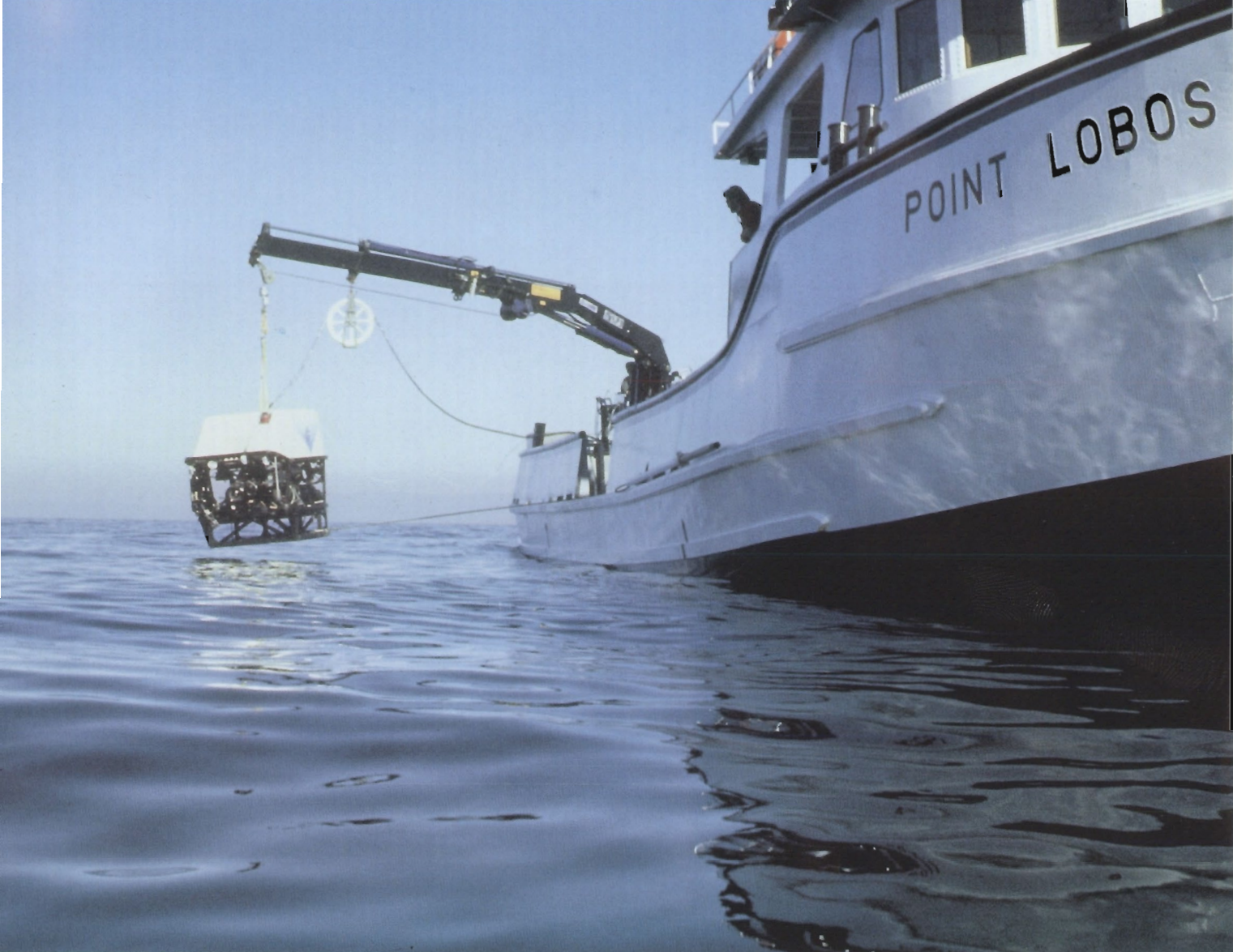
The Monterey Bay Aquarium Research Institute (MBARI) boat POINT LOBOS drops the remotely operated vehicle (ROV) overboard.
